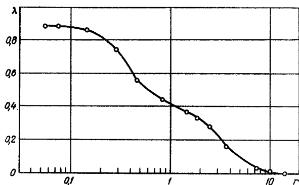
Fig. 1. Pore- (capillary) size distribution curve [ r is the pore radius in \mu ; the ordinates represent the ratio of the cumulative volume of the pores (of the same size) to the total pore volume; \epsilon_T = 0.302 ; \lambda_l = 4.0 kcal/h \cdot m \cdot ^{\circ} C; \rho_S = 3.93 g/cm ^3 ; unglazed alumina-based ceramic].
